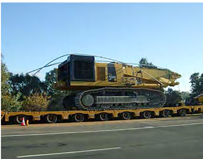
Oversized load that had to be turned back at Wagga Wagga and return to South Australia because of height restrictions on the rail-over-road bridge
